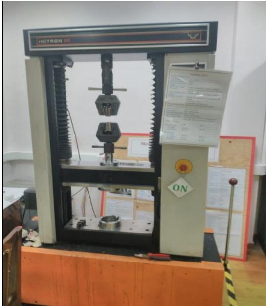
Figure 5(a) Front View of INSTRON 1195
