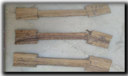
Figure 3: Fractured specimen after UTM testing
