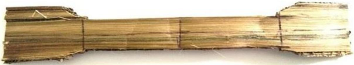
Figure 2: Original Specimen for testing using UTM
